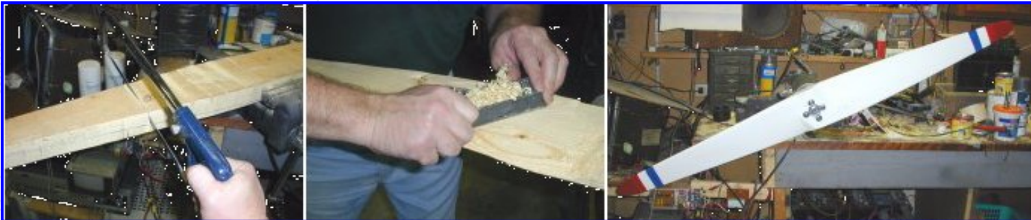
CARVING A WIND GENERATOR PROP Click on the photo to see the carving process
