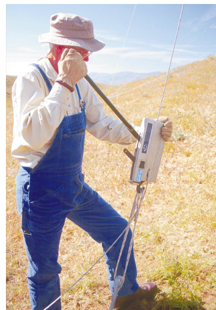
Below: Using the Super Pull-All to lower the tower. The cable passes through the body of the griphoist.
