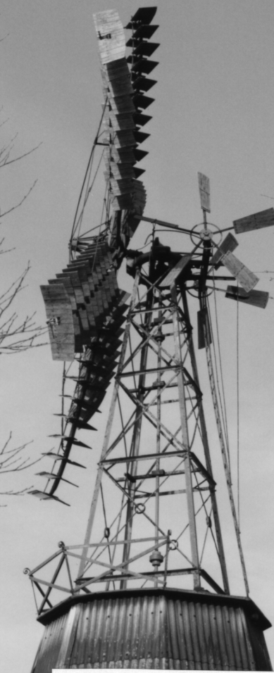
Wind machine for mechanical power, for farm or small factory use. Photographed in March 1994.
