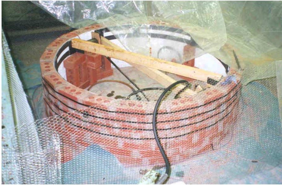
Figure 1 – Tests arrangement for externally reinforced brick cylinders
