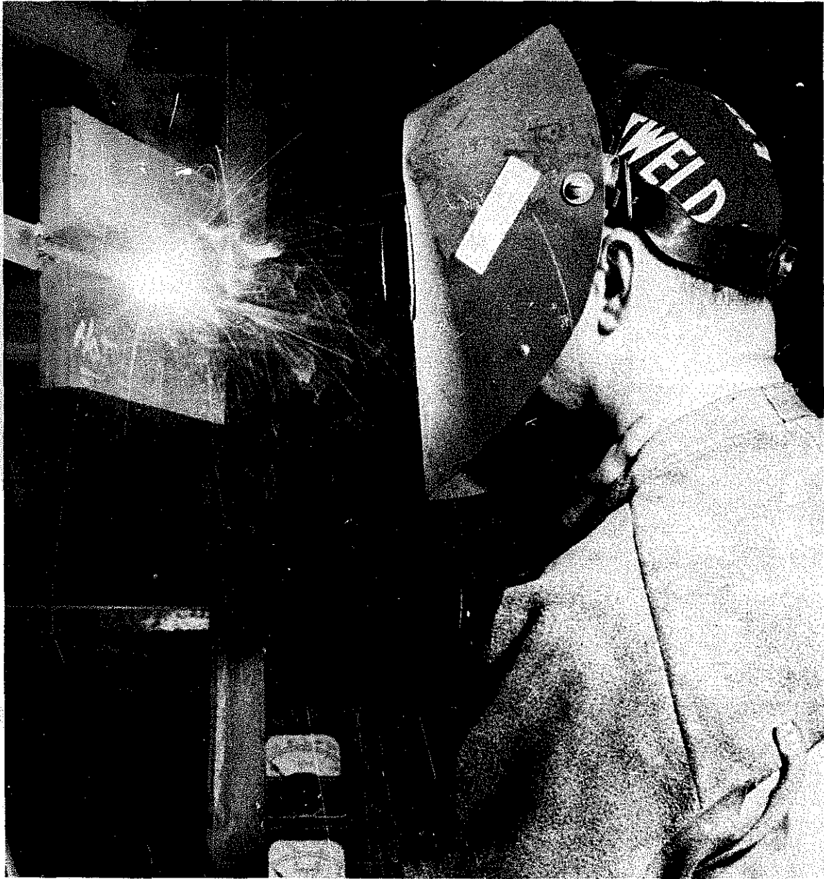
Weldor making a qualification test.
