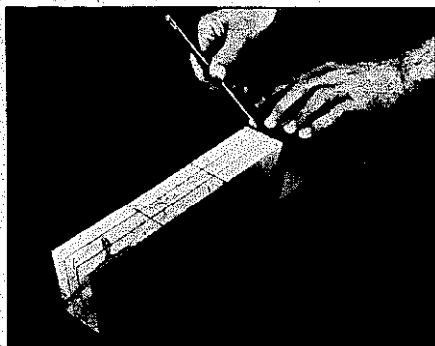
Mark the position for dowel holes on one piece, then line up pieces with the joining faces up and use a straight edge to carry the lines across the other pieces.
