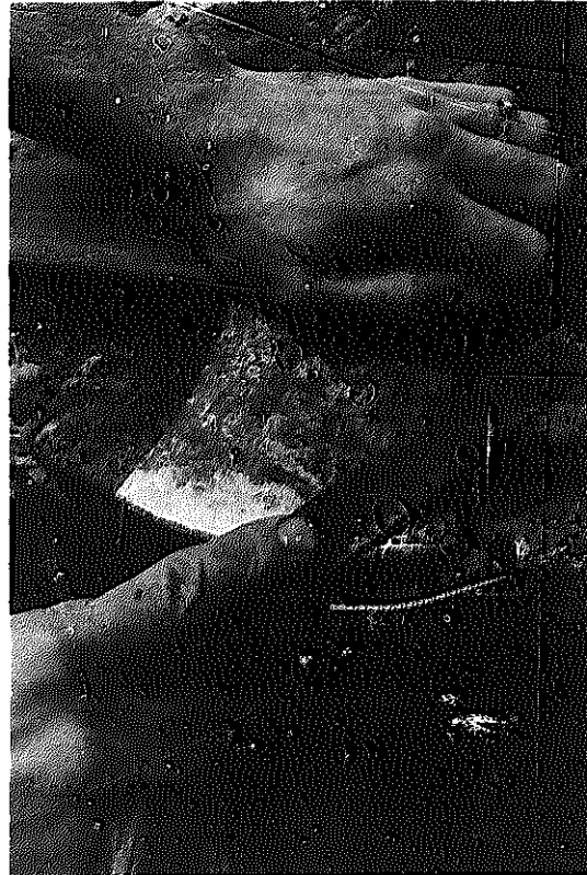
When sharpening the axe, use a full-size metal file. Make sure you do not sharpen the edge only, but work back one inch.
