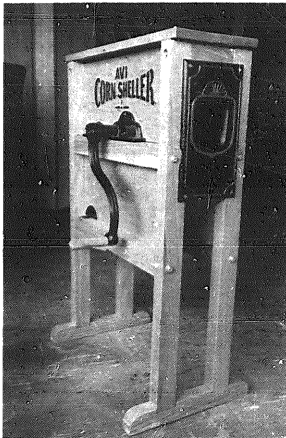
The AVI Cornsheller, showing the hand crank and corn exit. On the other side of the sheller, a large flywheel gives each stroke momentum.
