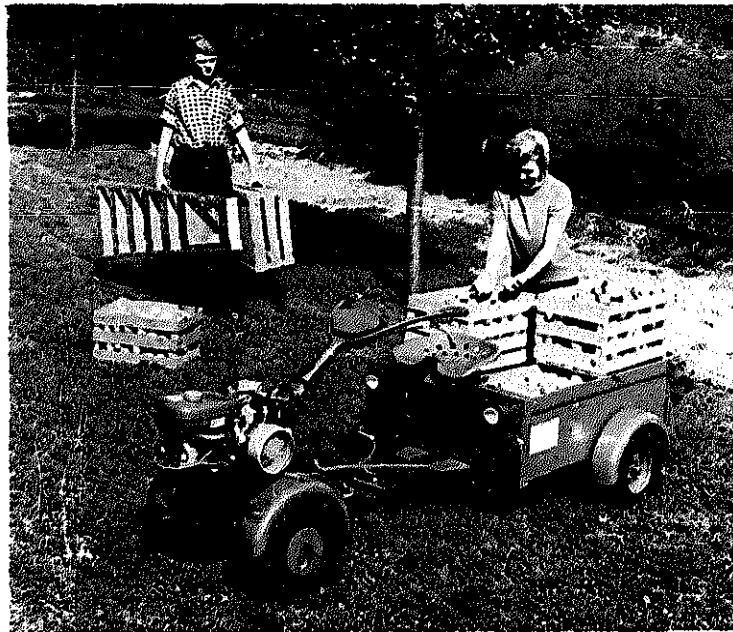
The Agria walking tractor with a hauling wagon, fully equipped for road travel. Agria-Werke
