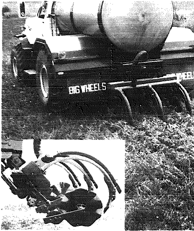
Big Wheels—a coultter/chisel combination to dig the application channel. Big Wheels, Inc.
