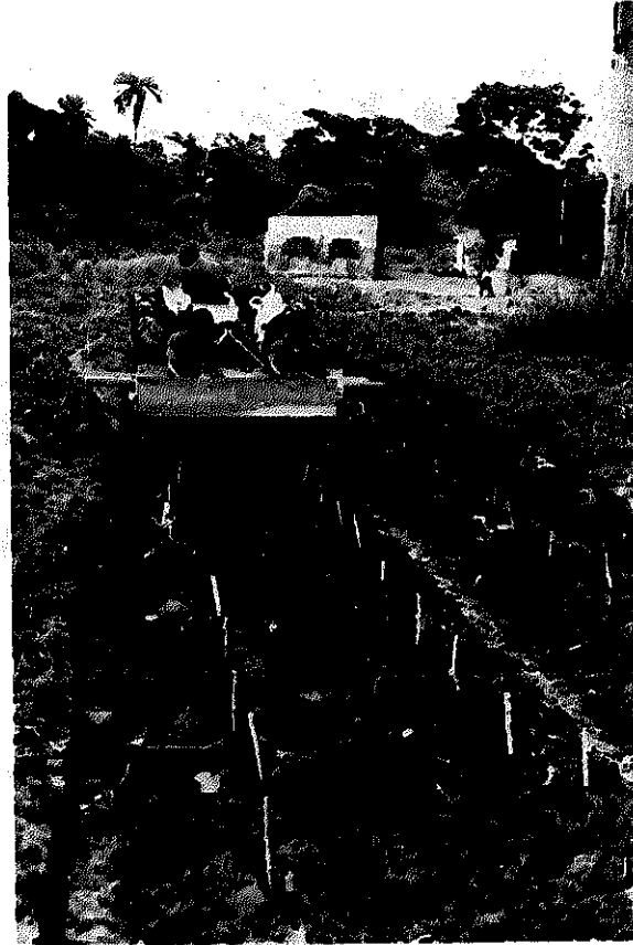
A two-row ridger in operation, pulling a planter behind it with a pipe joint.
