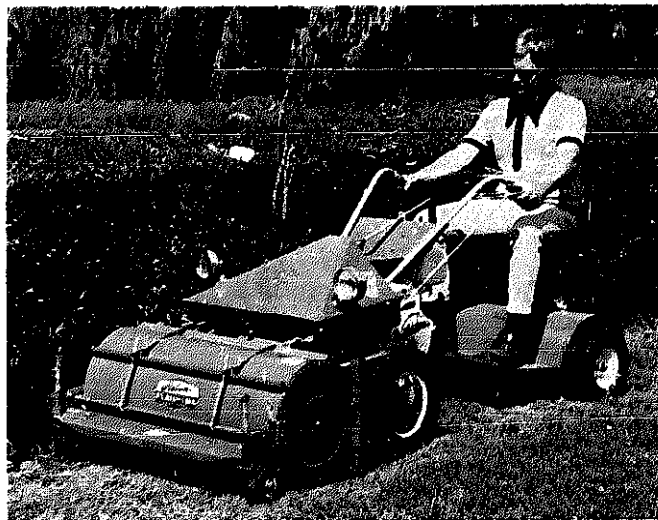
Haban's 12 h.p. self-propelled flail mower, complete with riding sulky. Haban Mfg. Co.
