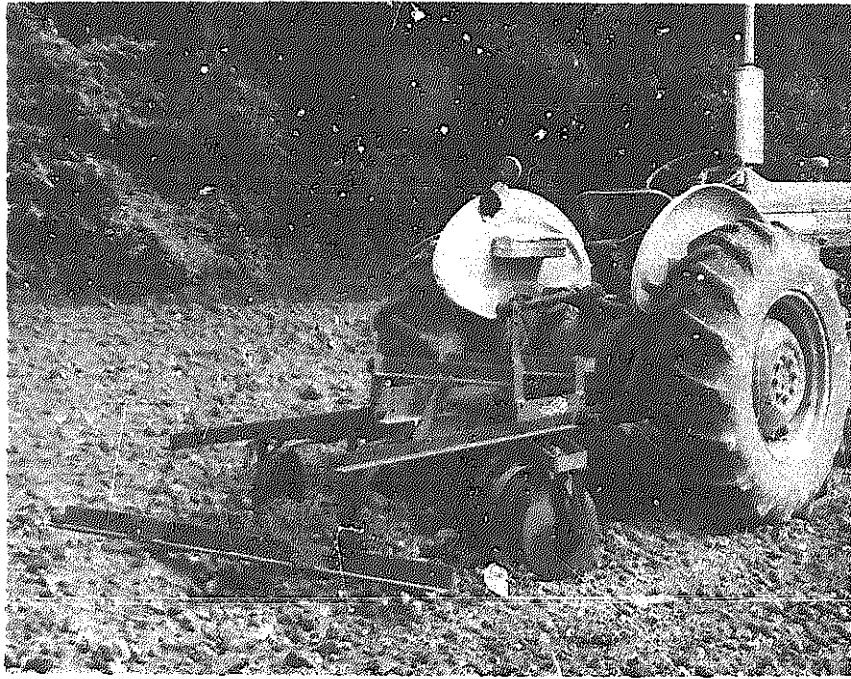
The Cole 510 system for chisel disking with four springs, center spring, six discs, and a smoothing drag for category 0 and 1 three-point hitches. Cole Mfg. Co.
