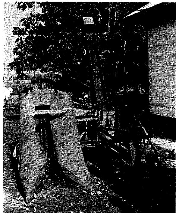
An old one-row, pull-type corn picker with a conveyor and PTO connection.
