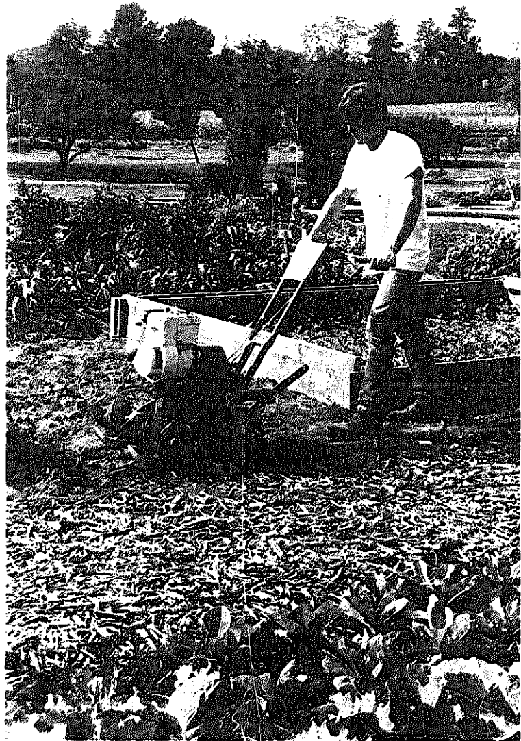
The rotary tiller earns its keep on the homestead by preparing garden beds in the spring, cultivating crops all summer long, and enriching the soil in fall with compost and cover crops.
