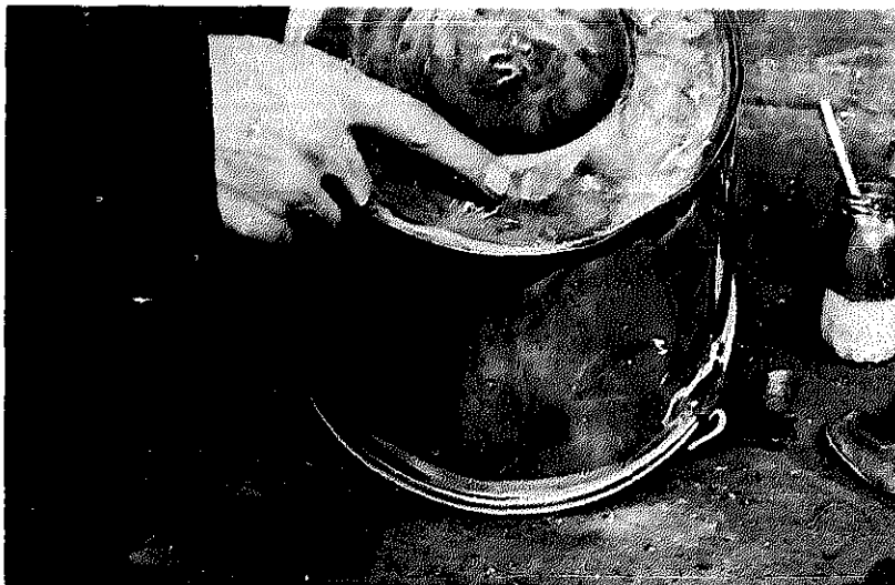
Fig. 18.7. Utensils with small holes may be repaired by soldering.
