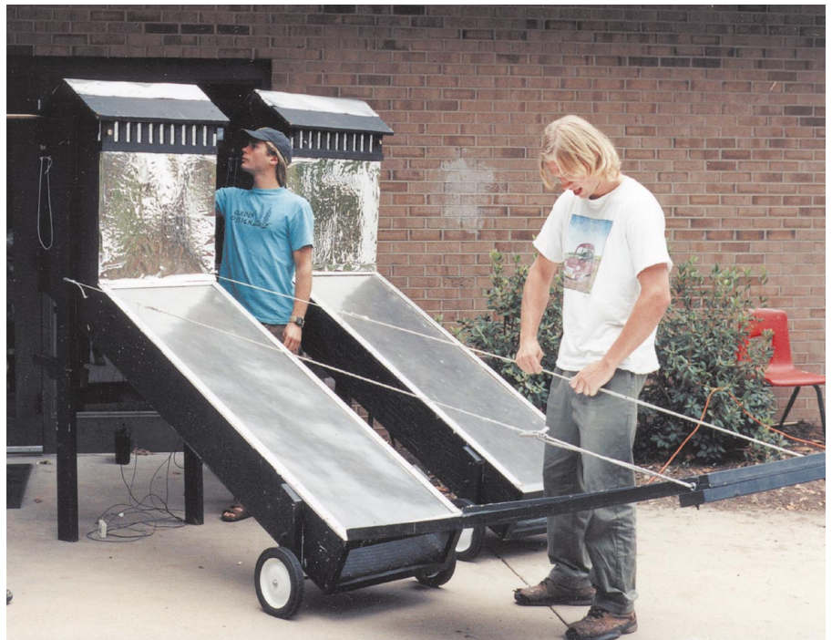
Above, Photo 4: Setting the front reflector angle.
