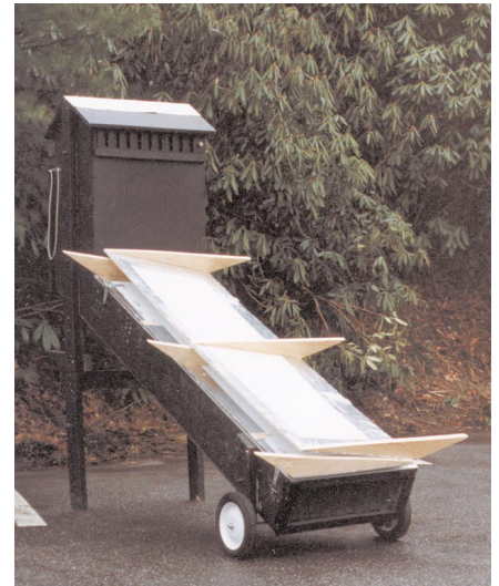
Right, Photo 5: Side reflectors folded onto glazing for transportation.
