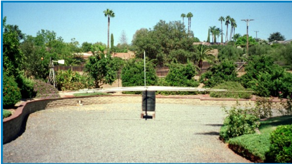
I used a Carpenters bubble level with a riser block on each side to verify that all elements were in plane. (Level not shown)
