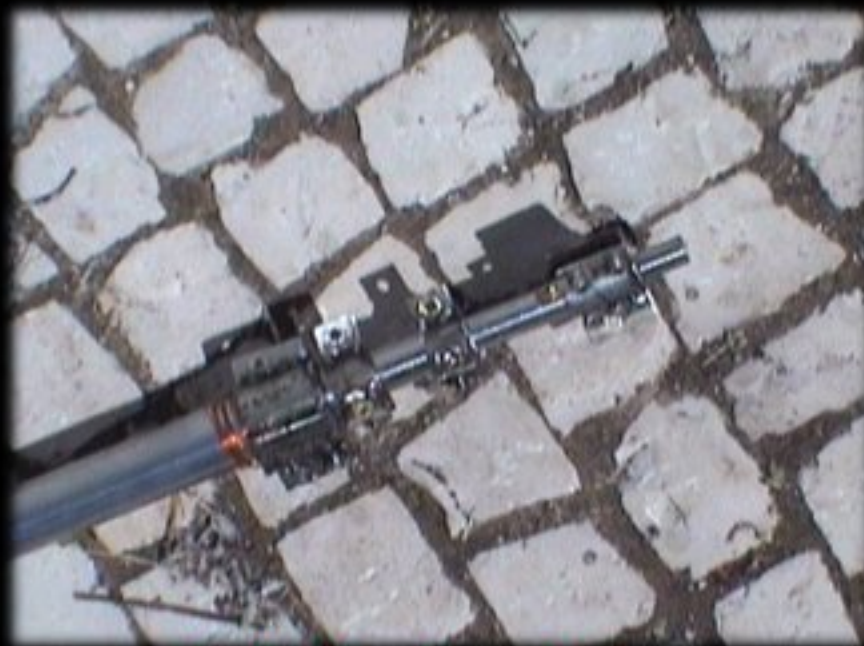
Details of the telescopic antenna sections with guying clamps.
