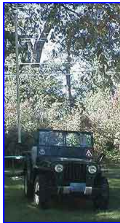
The 10-foot tall, two-inch diameter IFA antenna on N9ZRT's jeep. [N9ZRT Photo]
