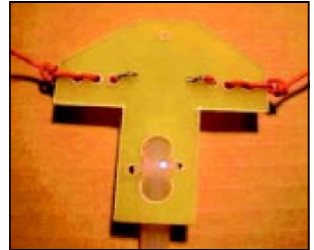
Figure 5—Here the feed-line-to-tuner connector is shown attached to the binding posts of the Squirt antenna tuner.
