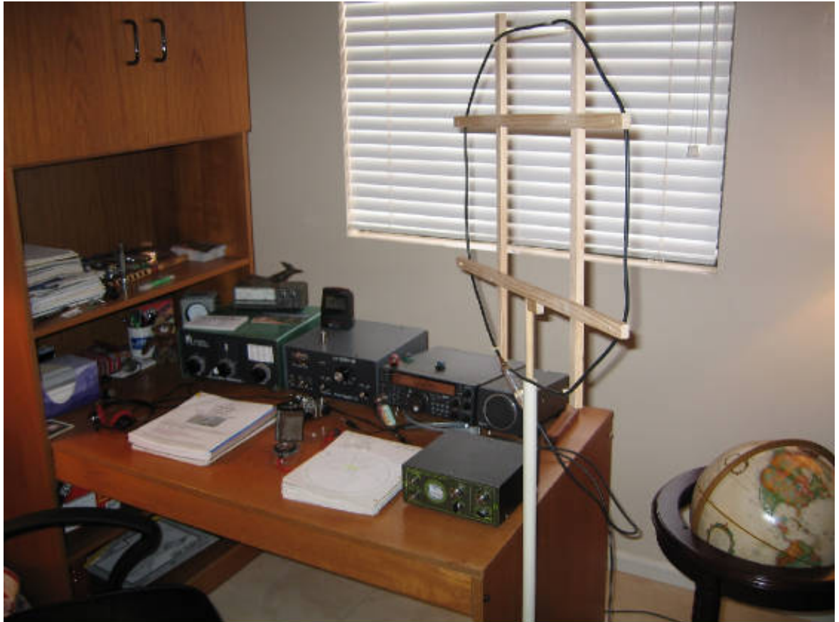
20m HF Receiving Loop Antenna
