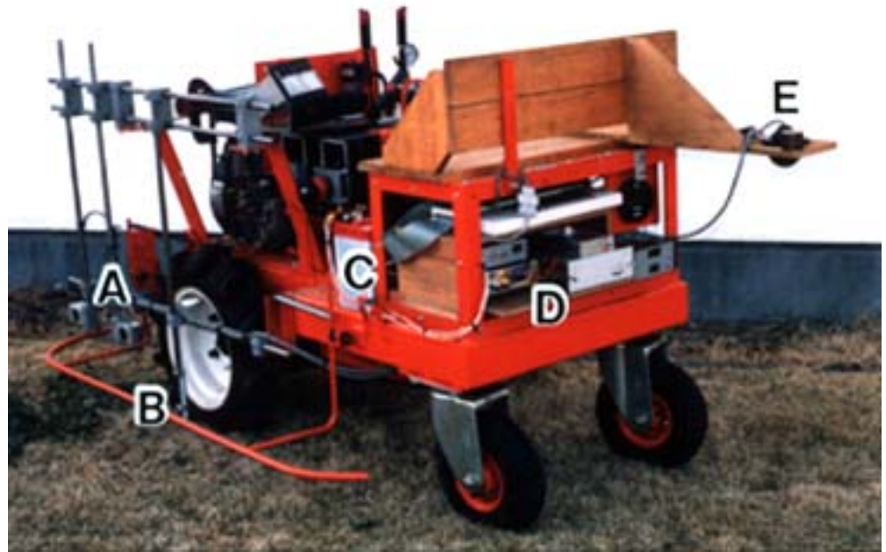
Fig. 8. Experimental vehicle equipped with steering control system
