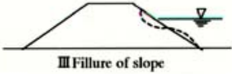
Fig.5. Classification of damage types
