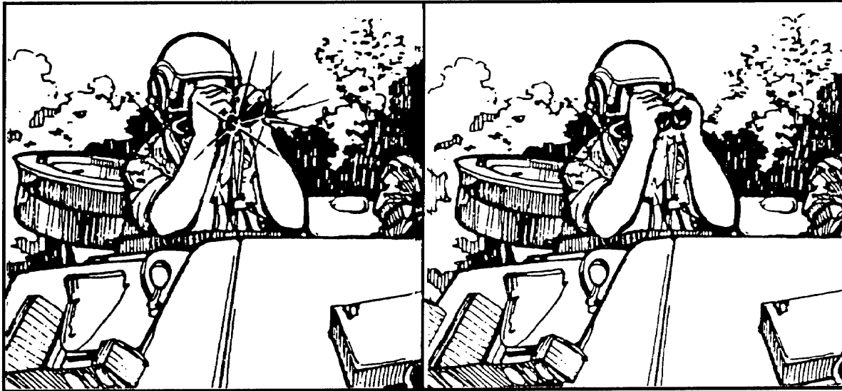
Figure E-1. Shade optics to prevent shine.
