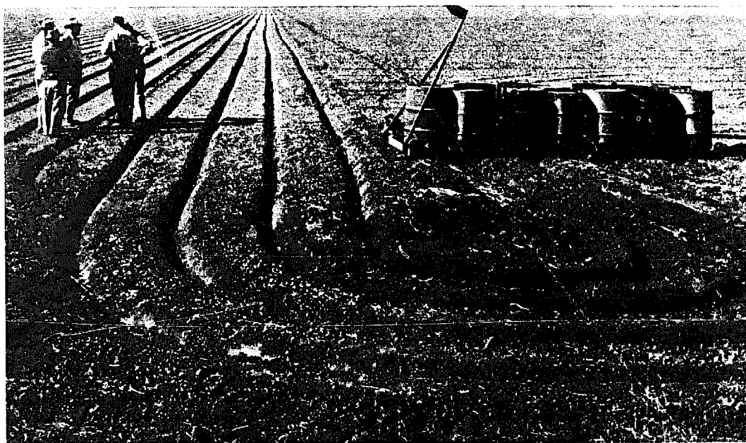
FIGURE 79. Corrugations which have been pressed into the soil by the corrugator (on right). Barrels filled with water add the weight needed to form the indentations in the soil. These corrugations will be used for irrigating pasture on flat land.
