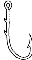
Fig 108 'Sliced hook' for fixing special bait.
