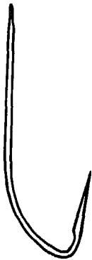
Fig 203 Sturgeon hook from the Black Sea. Between point and bend the hook has a thickening like a barb to prevent the rope with the float attached, (Fig 201a) from slipping over the point.
