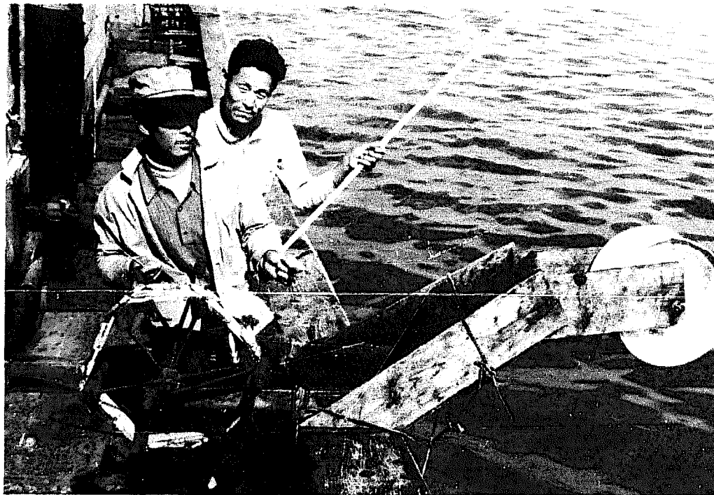
Fig 212 Korean squid fishing: ( behind ) older form with pole and line; ( in front ) newer type with hand-operated jigging machine (1972).
