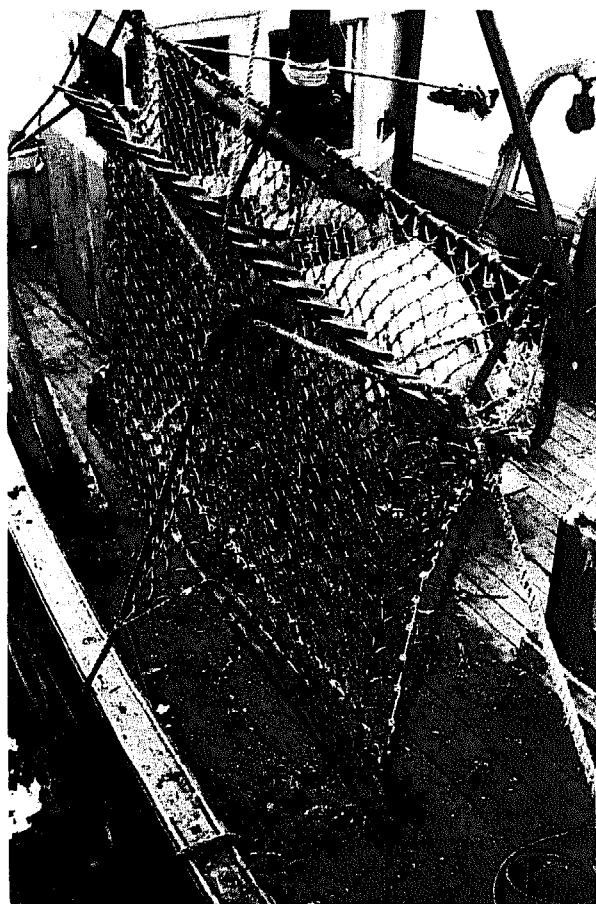
Fig 456 French dredge, Dutch type, with teeth for the collecting of venus-shells. (Photo: R Piboubes, Brest.)
