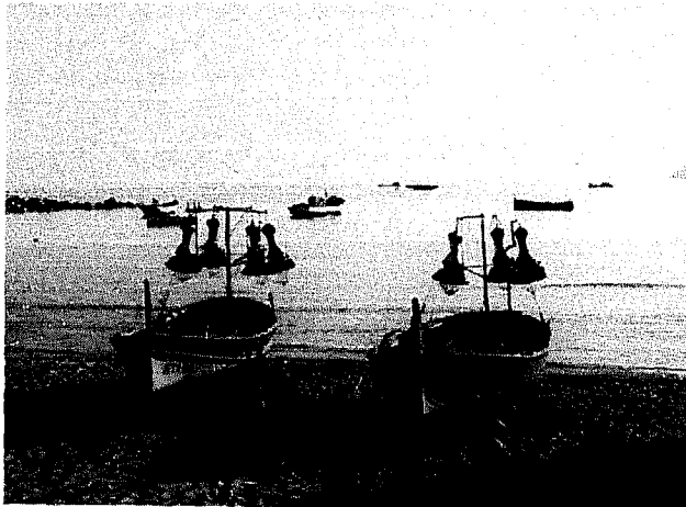
Fig 175 Spanish boats of Benidorm equipped with powerful lights for attracting sardine. (Photo: J Schärfe.)
