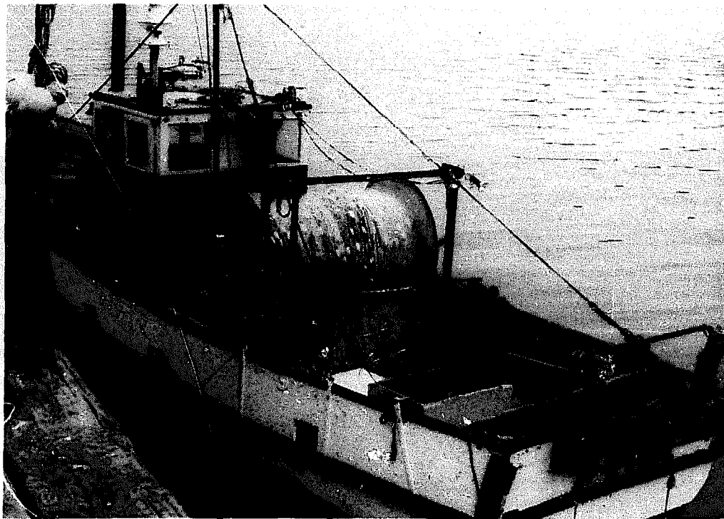
Fig 688 Gillnetter with a large shark net on a drum in the harbour of Akaroa in New Zealand (1981).
