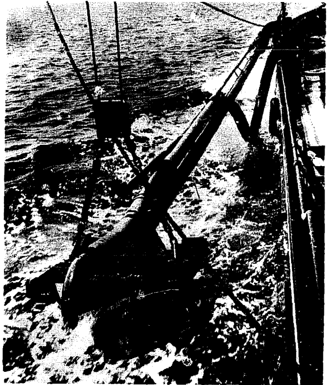
Fig 725 Dredge with high pressure hose and larger suction pipe of a British cockle dredger. (Photo: Meixner.)
