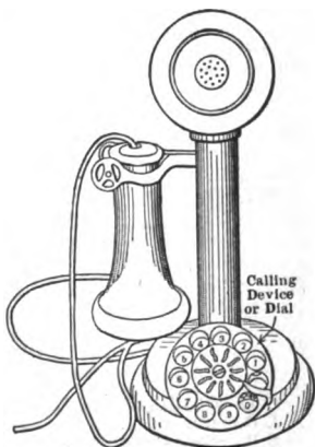
FIG. 27.—Desk stand equipped with calling device or dial for automatic (Strowger) service.
