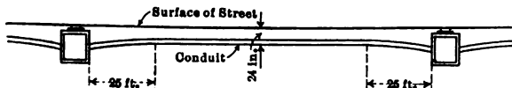
FIG. 68.—Section of underground conduit showing method of grading for drainage of ducts.
