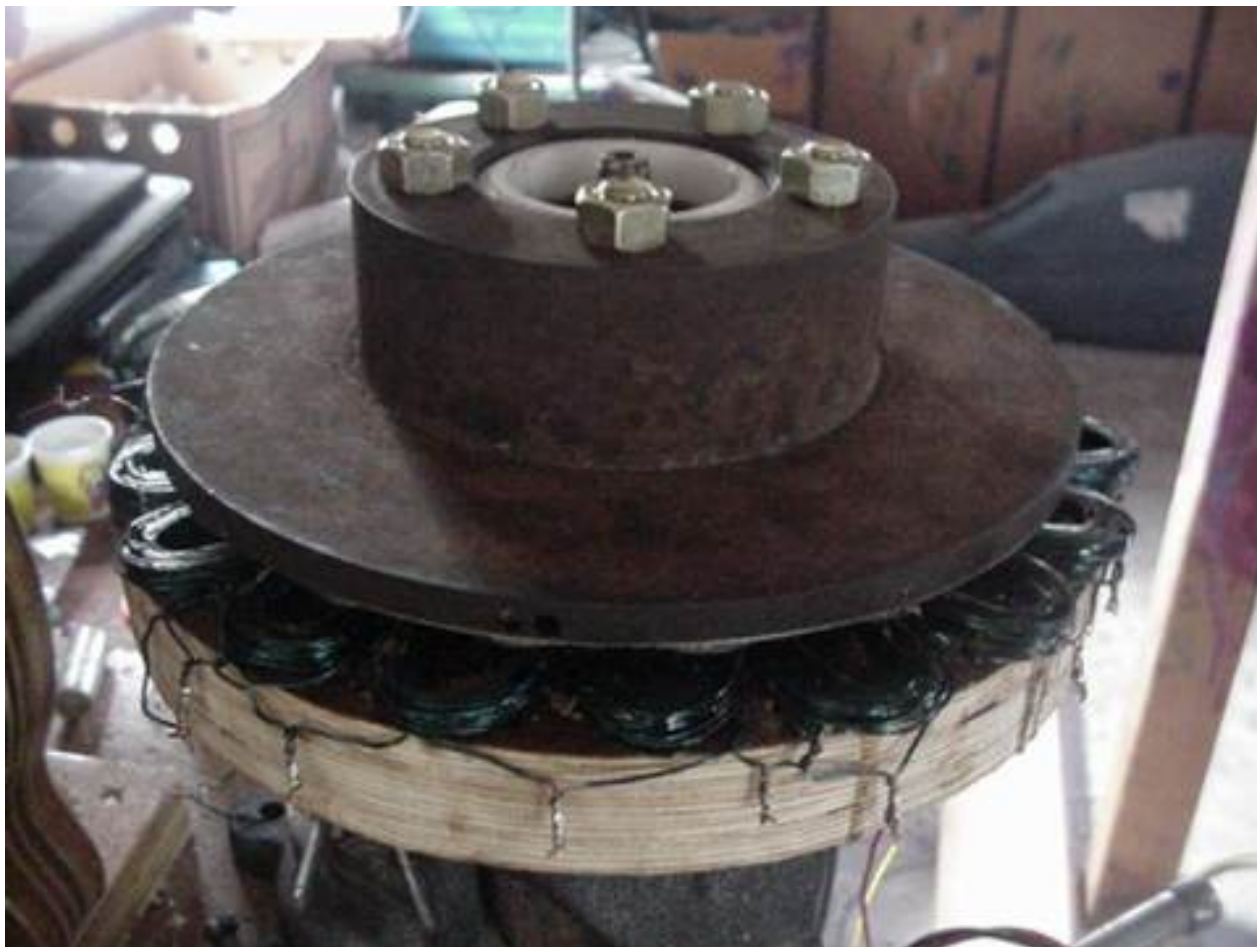
Homemade Volvo Brake Disc PM alternator, 800 watts, $150!
