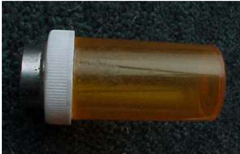
Float with magnet glued on top
