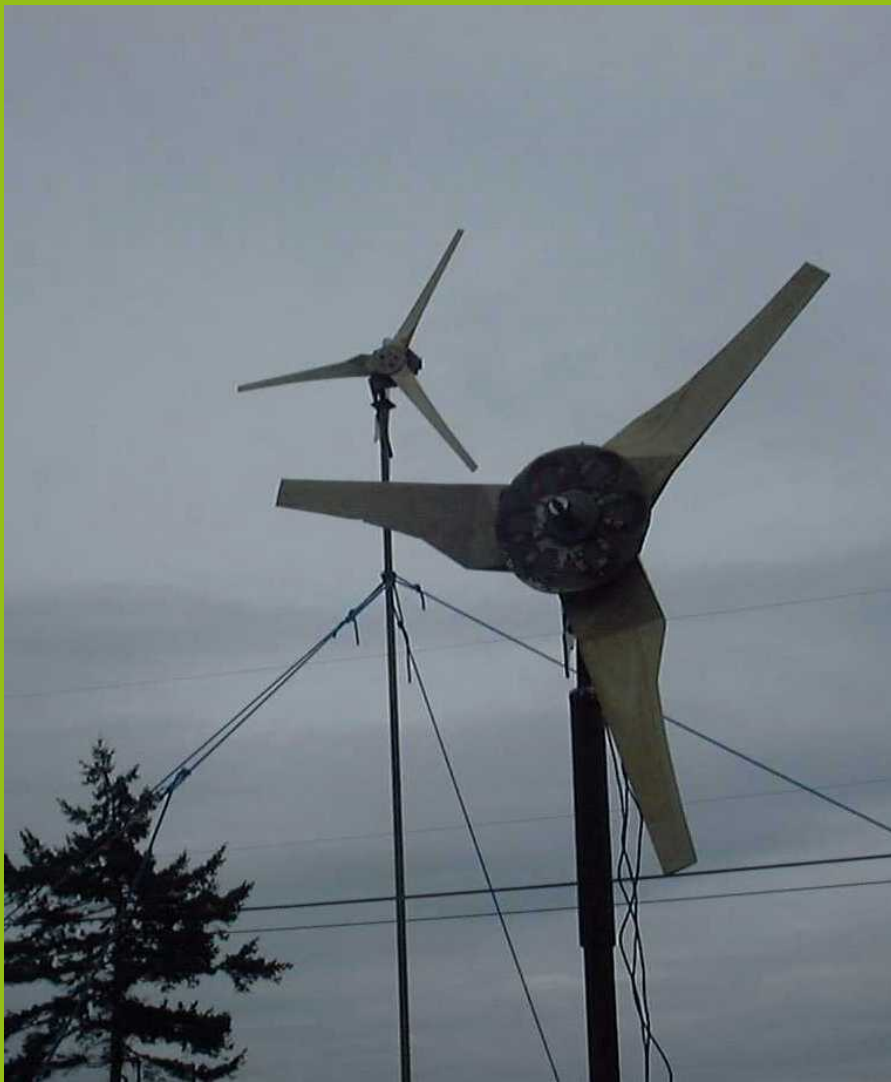
The big machine is on the tall tower (twenty feet up but still not nearly tall enough) and the little 4' diameter machine is on a short stand in the foreground.
