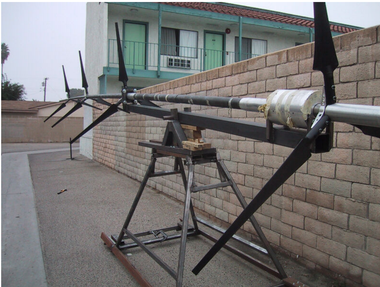
View from region of generator - 3 kW prototype Selsam Multi-rotor wind turbine partially assembled on stand at ground level
