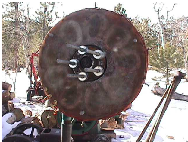
Above is shown the stator. In this alternator, the back rotor is mounted well behind the hub, so that the wheel hub is actually centered in the stator. The studs between the two rotors are very short, and strong (I hope!).
