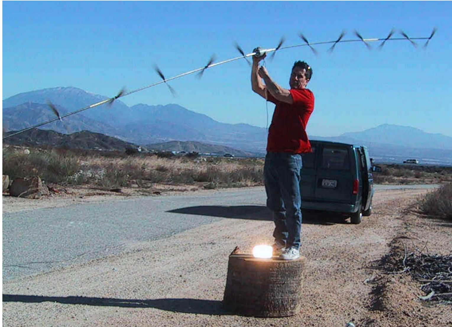
The car headlight at Doug's feet is 50 watts The rotor size is only fourteen inches! Wind speed in the 20's mph (more rotors produce more power)
