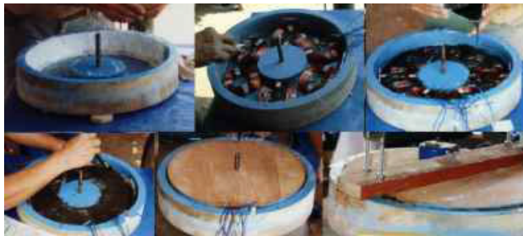
Six stages of the rotor casting procedure
