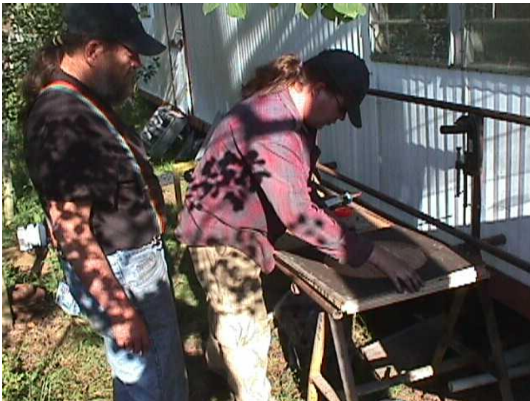
DanF and Tom are working on the mold. It's basically a 3/4" piece of plywood 18" square, and on top of that we have 1/2" material with a hole 14" in diameter in it. In the center of the mold there is an island (Aslo of 1/2" material) 5.5" diameter. I think next time we'll reduce that to 5", as it would fit around the studs and make the coils fit a bit better. This worked fine though. The lid for the mold is simply a disk of 3/4" plywood 14" in diameter.
