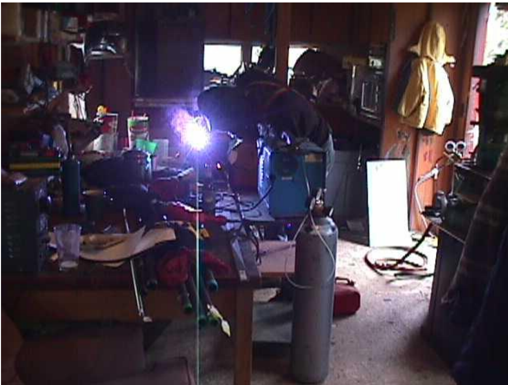
We cut the strut so that the spindle could be welded to the side and offset from the tower about 5". Pictured above Tom is welding all this together.
