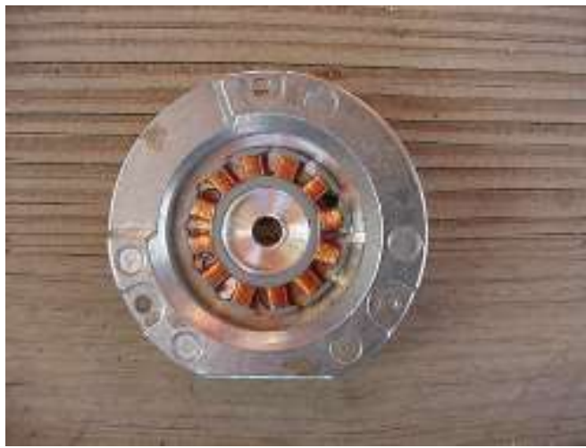
Internal coil layout of the brushless DC PM motor
