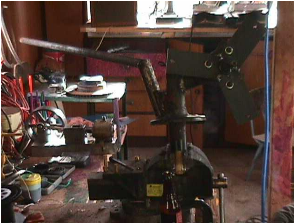
Pictured above the main chassis of the wind turbine is pretty much together. You can see now how the stator bracket bolts on.
