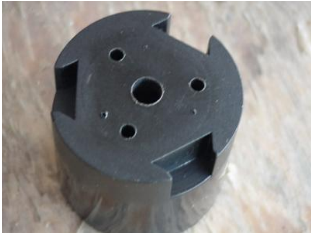
Completed anemometer hub assembly
