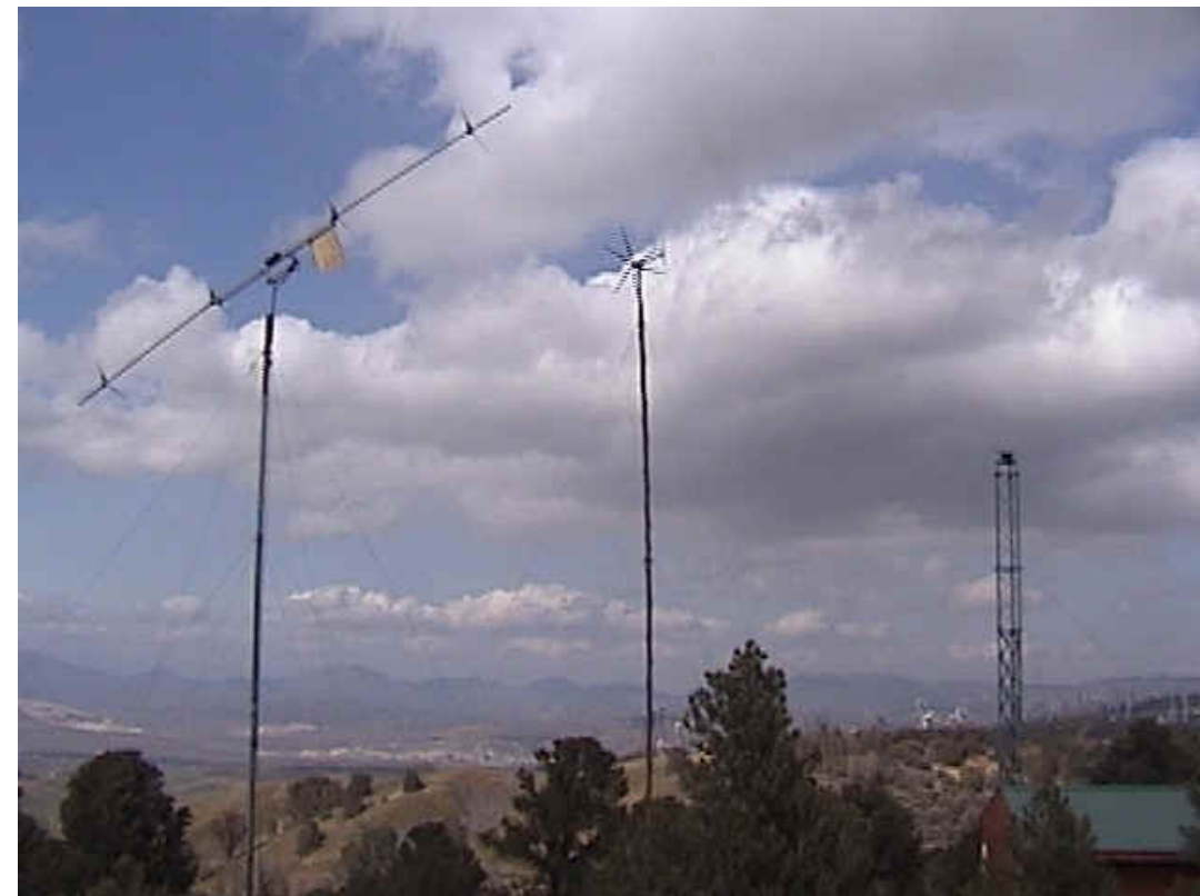
Experimental Prototype Selsam Wind Turbine with four 4-foot diameter rotors (left).
