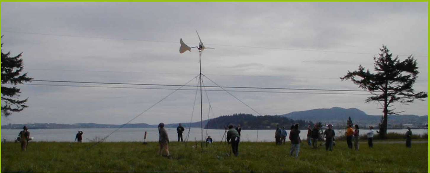
This is the bigger of the two machines we finished during the course. Rotor diameter is 8 feet (2.4 metres).
