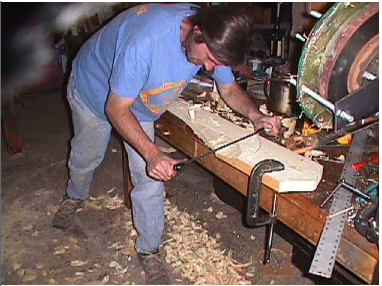
Pictured above we are roughing out the front of the blades with the draw knife.
