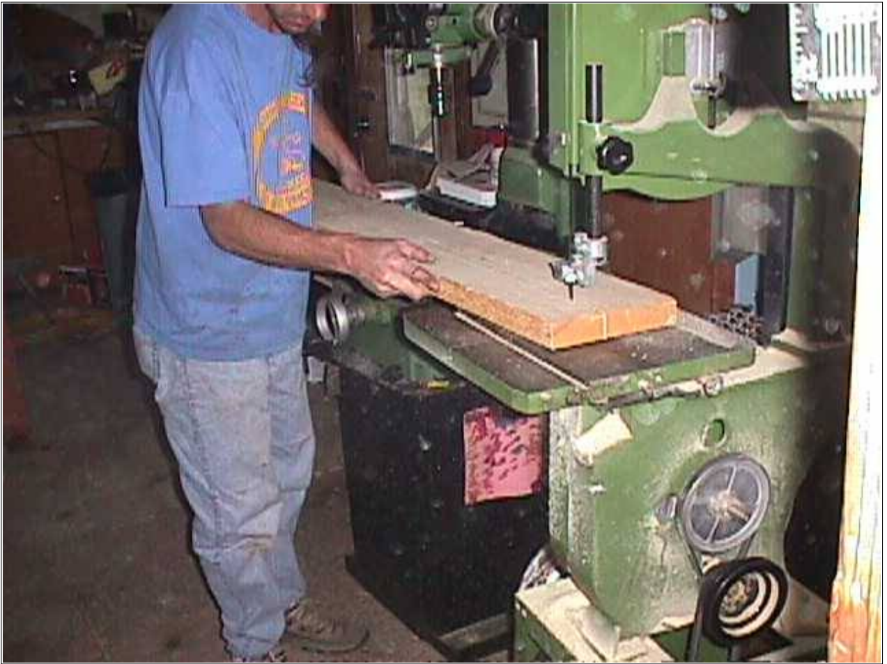
Here Dave is cutting out the blades on the bandsaw.
