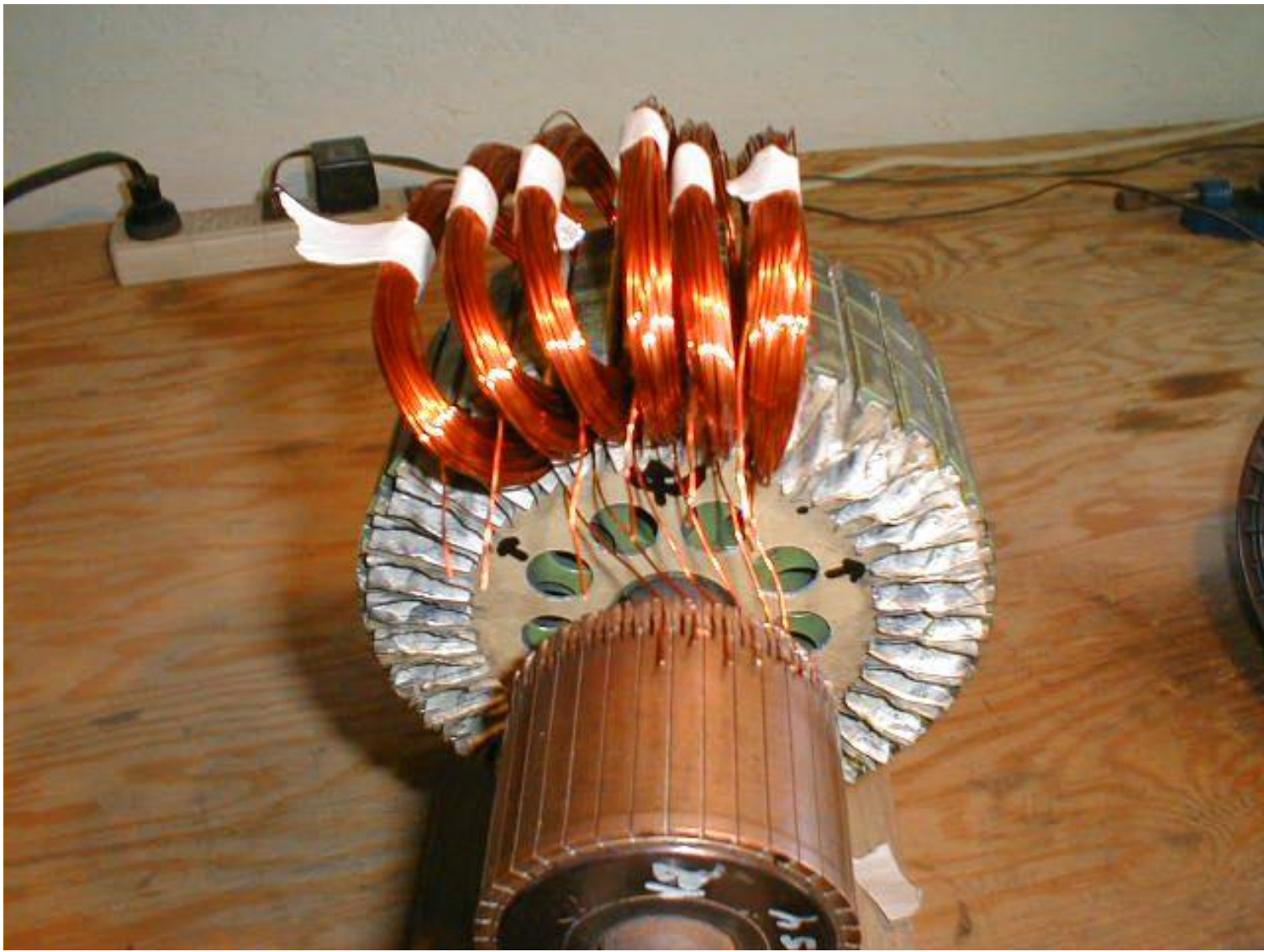
The first six coils, lower ends installed. Tape secures the coils until they are installed in the slots.
