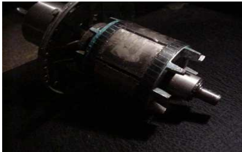
Armature converted with permanent magnets
