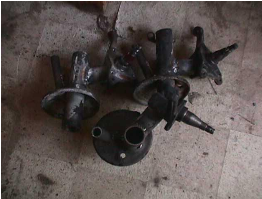
Pictured above we have 3 main windmill frames welded up. You can see how the tail pivot is angled at about 20 deg.
