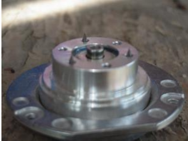
Nails in motor for marking hub holes.
