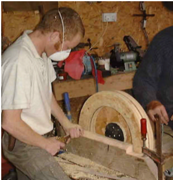
Turning a stator mould on an electric motor
