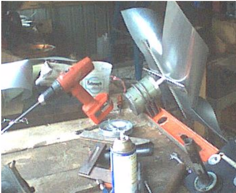
Rear of pinwheel assembly showing the support pieces of aluminum strap.
