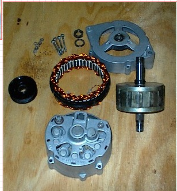
One of the original alternator modifications. This one had a rewind stator and the modified rotor using Neo' magnets.
