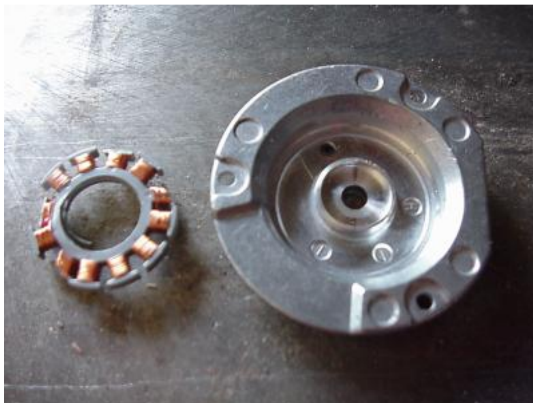
Coils removed from Motor
