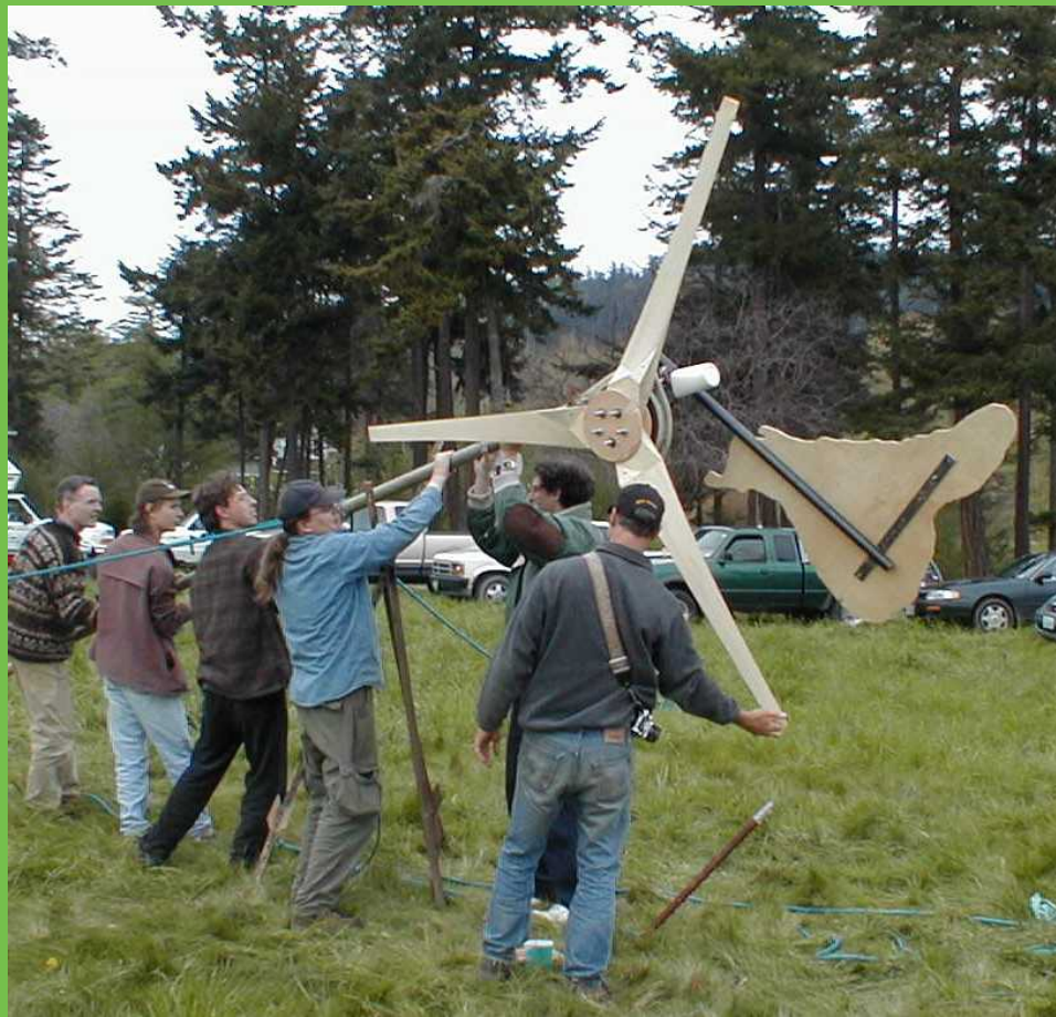
The large one has an eight foot diameter rotor and 500 watt output. The smaller one (below) is half the diameter and one quarter of the output. We only use a single magnet disk on the smaller machine.
