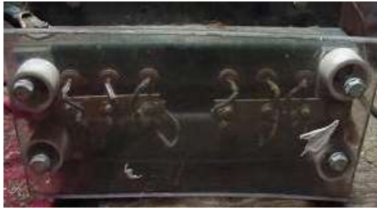
Close up of home built diode bridge
