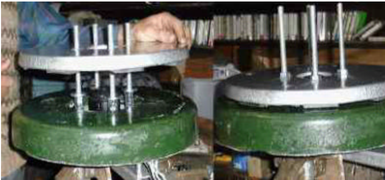
Fitting the front magnet rotor
