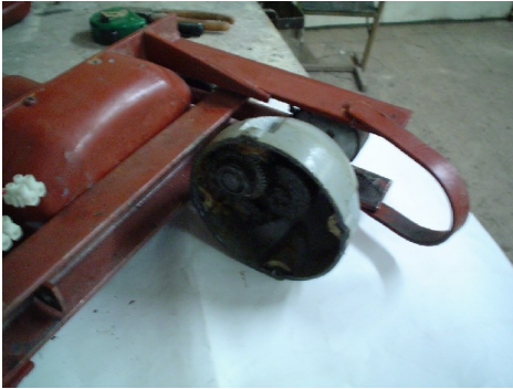
Gear box ( ratio 1:6)
