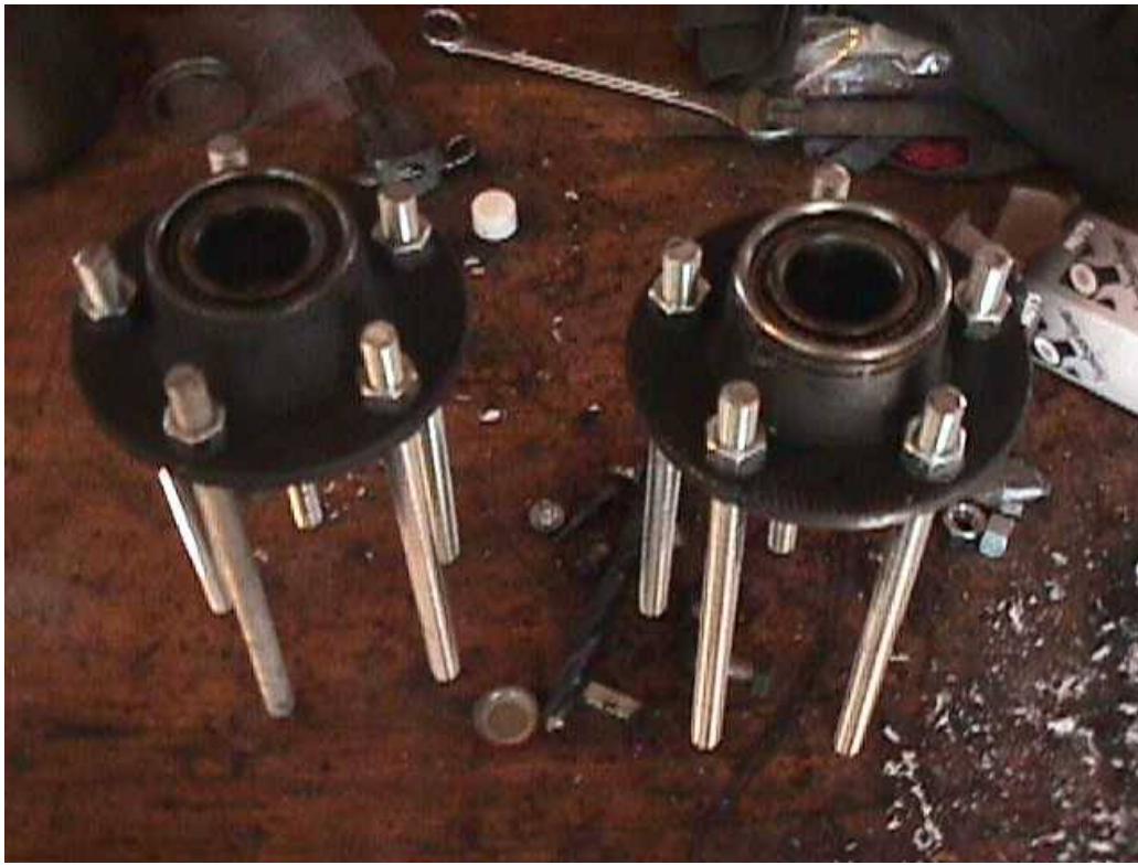
The studs are replaced with 10" pieces of 1/2" - 13 allthread.
