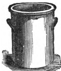
FIG. 43. DIPPING OR MIXING PAN FOR ACID PICKLES.
