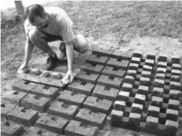
15-6 Production of special adobes
