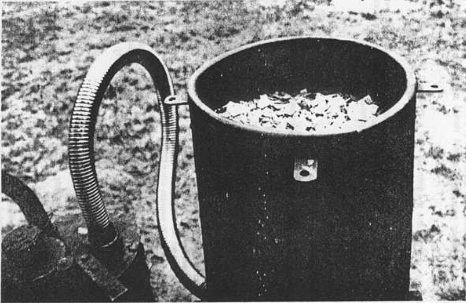
Fig. 3-1. Virtually all varieties of wood chips can be used for fuel. (Minimum size for this 6-in. firetube unit: 3/4 by 3/4 by 1/4 in.; maximum size: 2-in. cubes.)
