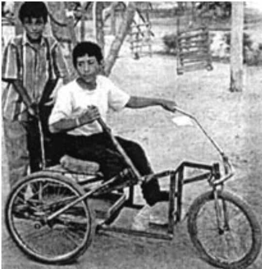
The front steering mechanism uses a fork made with strong metal tubes. The front wheel is a 24-inch bicycle wheel.
