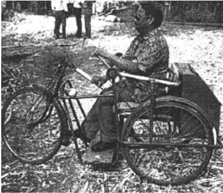
One of the participants in the UN workshop tries out Ram's tricycle. Hand-pedals that power both rear wheels make it an "all terrain vehicle."
