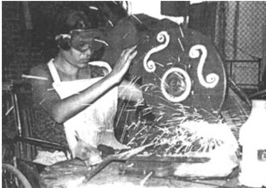
Maria de Jesus, who is paraplegic, cuts a metal tube for a wheelchair she is making in a training workshop at PROJIMO.
