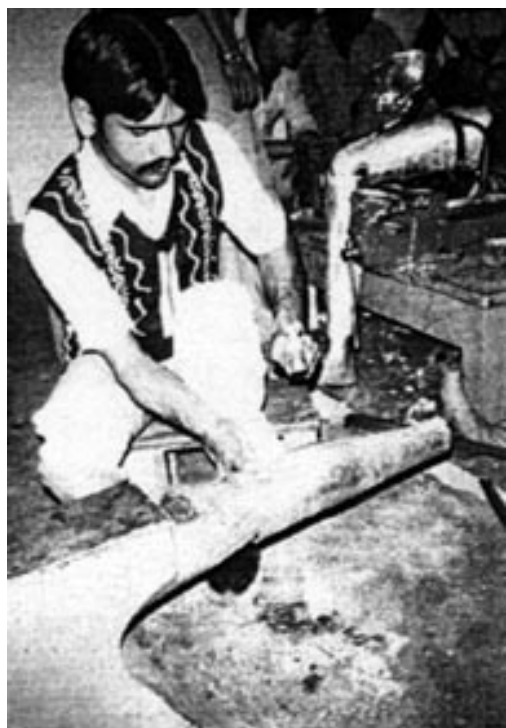
He hammers the tube to look like a leg and to correctly fit the stump.
