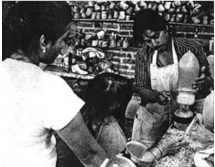
A young woman watches Marcelo and Conchita make a fiberglass-and-resin socket for her artificial leg. This modern technology is done at the small village center, at relatively low cost (less than one fifth the cost she would pay in the city).
