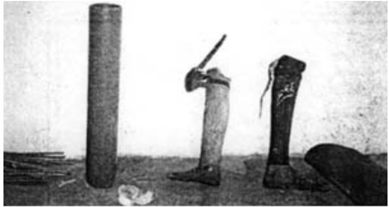
Plastic pipe is converted into prosthetic legs, as shown here.
