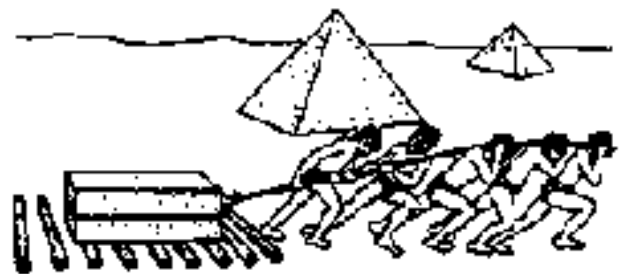
Rod bearings were used to move the rocks to build the pyramids in Egypt.
