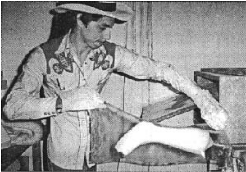
Marcelo drapes hot plastic (heated in the oven, at right) over the plaster mold of Carla's foot, to make a brace.
