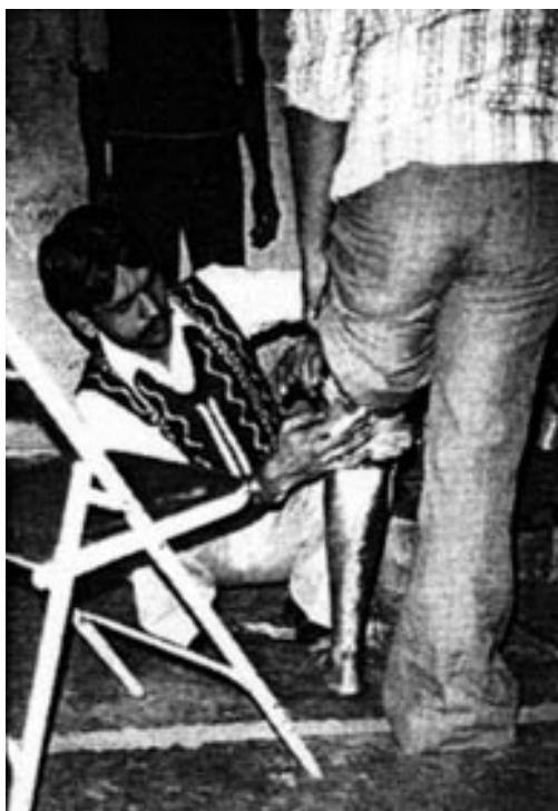
After attaching the foot to the tube, he adds padding and a strap, and tries it on Gopi's leg.
