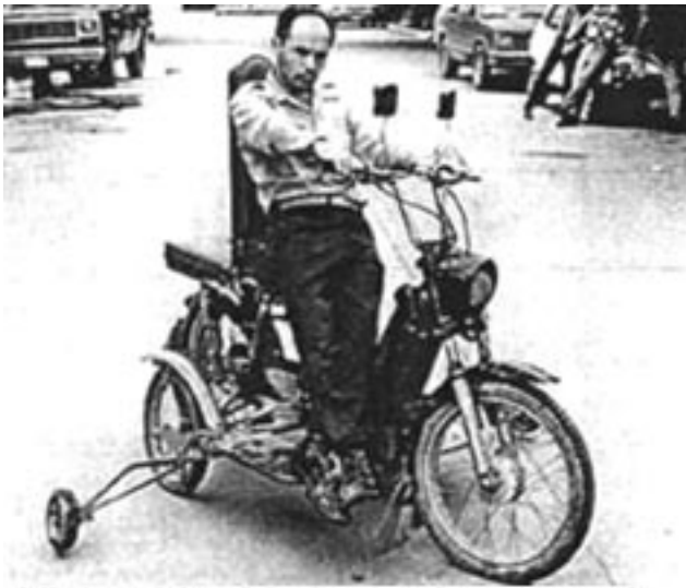
Victor rides his 6-wheel motorcycle. The small "out-rigger" wheels keep his jerking body from upsetting it. He removes them to pass through narrow doors.
