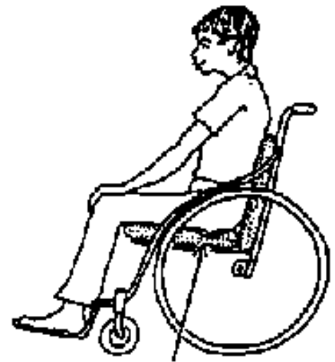
Cushion placed correctly.
