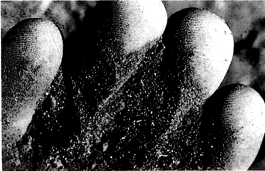
FIGURE 47 . . . in this soil from the same pond after treatment sodium carbonate has caused the clay aggregate to break down into fine particles that retard seepage. . . .
