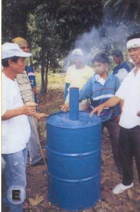
e. Modified drum kiln can be used for charring shells, husks, wood pieces and corncobs.
