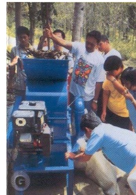
f. The metal plate carbonizer is a simple low-cost machine capable of carbonizing not only sawdust and rice hull but also coconut coir dust and other carbonaceous fine materials.
