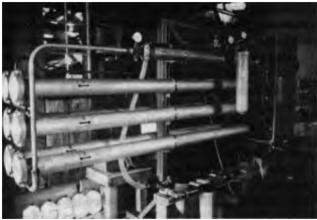
Reverse osmosis system for making maple syrup. Photo courtesy of Paul Sendak, USDA Forest Service. (SFP-6)
