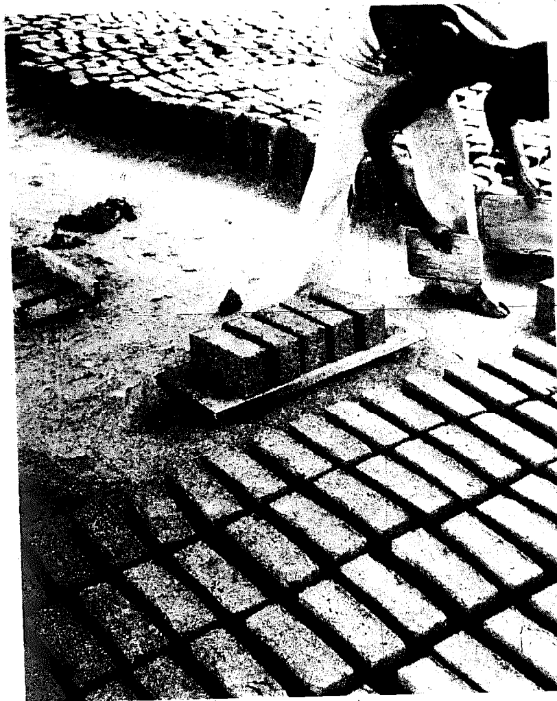
Accurately sandmoulded bricks set out for initial drying. In the background, bricks are upturned to avoid drying distortion
