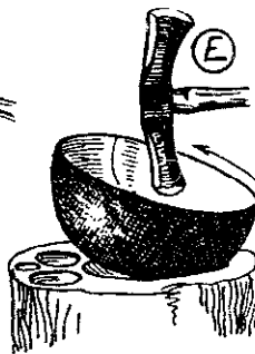
Work the bottom right in to centre
