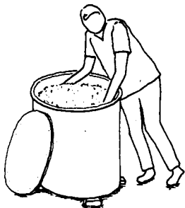
Take the intermediate trays with the used absorbent out of the chamber.
