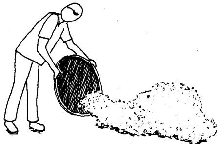
Throw the absorbent onto the ground.
