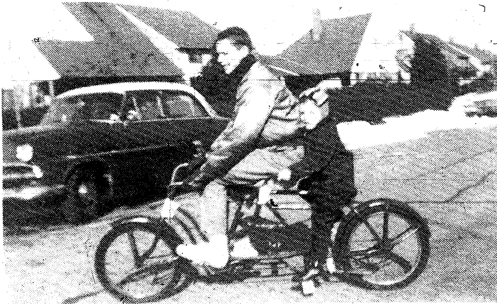
Fig. 13-3. A tandem built by joining two frames together.
