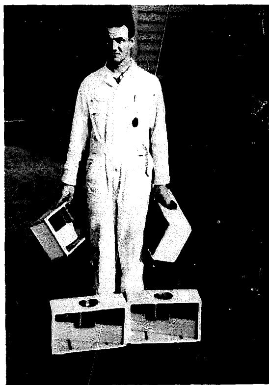
These cages with solid ends are a much stronger construction than those with open ends, and are the type generally used.
