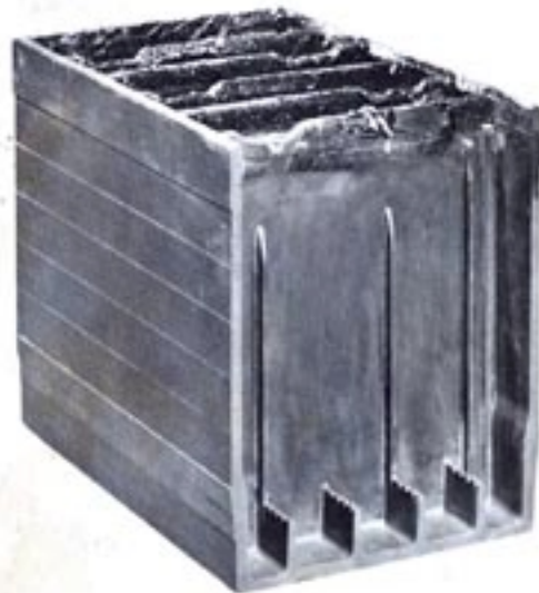
Fig. 38—Element rests severely-notched by vibration of loose element or battery loose in hold-downs.
