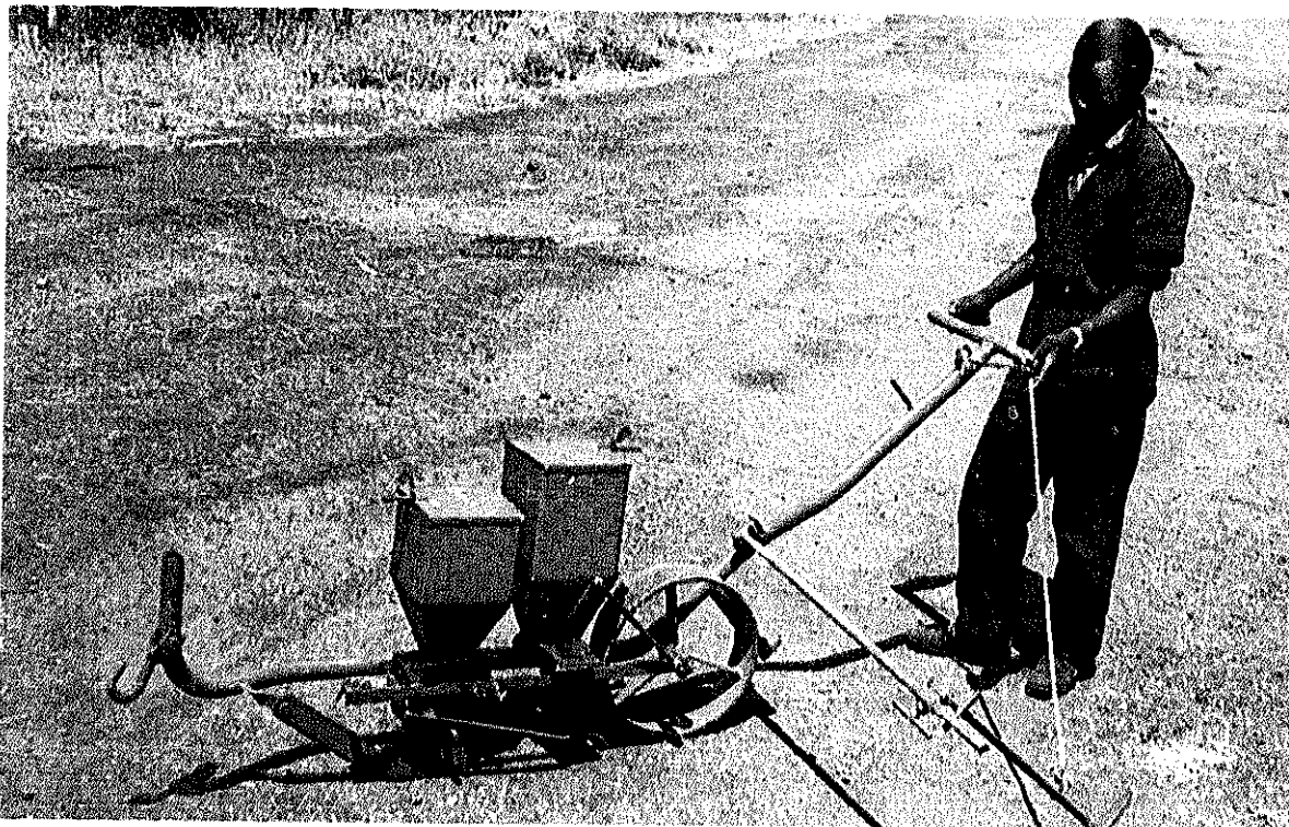
Fig. B/II/49 : Seed spacing planter with mineral-fertilizer placement attachment. The fertilizer is accurately placed near the seed, e.g. as deep fertilizing for maize. (TAMTU, Tanzania)
