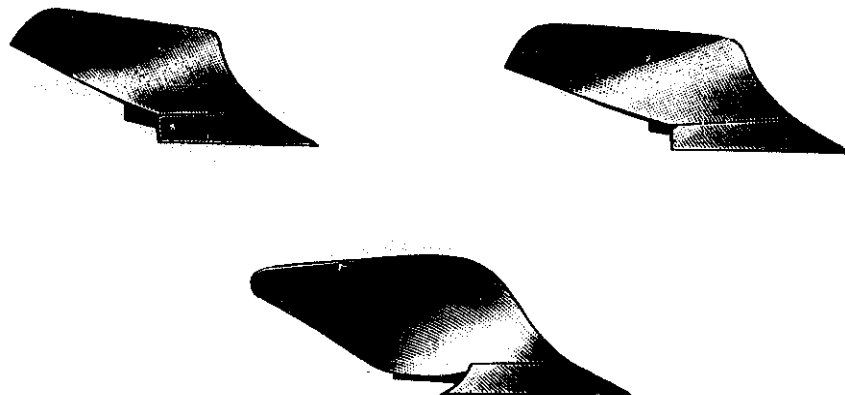
Fig. B/II/21: Plough bodies (VENTZKI) Top left: continental body Top right: general-purpose body Bottom: semi-digger body
