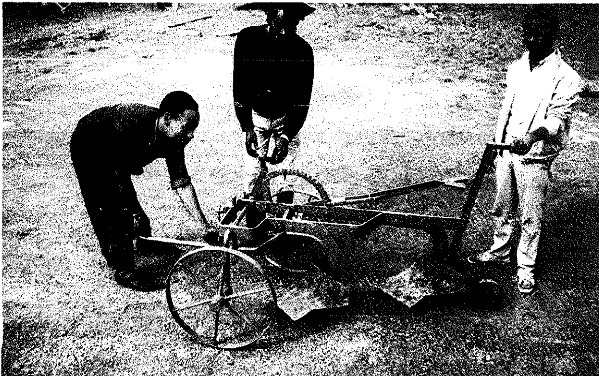
Fig. B/II/26 : Two-furrow frame plough. The third wheel behind the second body is required only for transporting the plough. (TAMTU, Tanzania)
